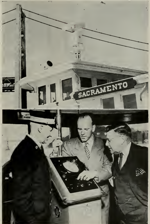
The Radar rotating ("whirling eye") antenna on top of the Southern Pacific ferryboat Sacramento. The rotating antenna is analogous to a rotating searchlight in that it sends out radio beams to locate obstacles in the ship's path.
